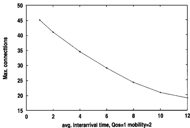
Fig. 12. The maximal number of connections for QoS<sub>1</sub> traffic.
