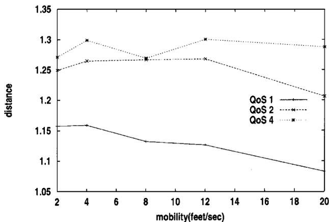
Fig. 14. The average value of  $d$  for different QoSs.
