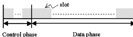
Fig. 1. TDMA time frame structure.
