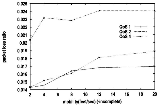
Fig. 13. The average packet loss for "complete" connections.
