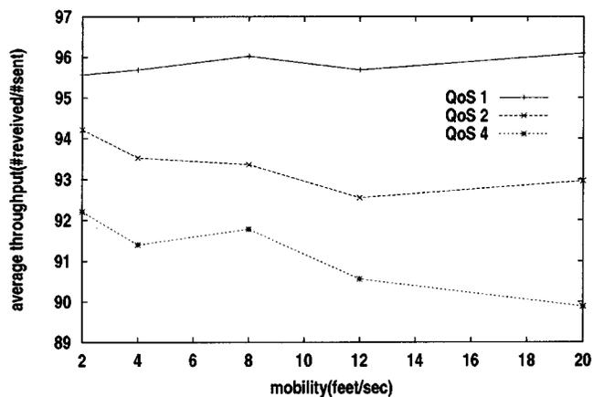
Fig. 8. Average throughput (%) of different QoSs.
