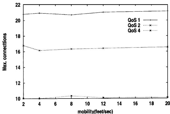
Fig. 11. The maximal number of connections.
