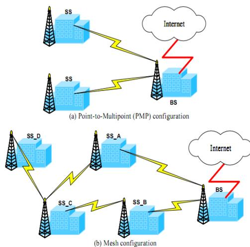
Figure 1. Two Configurations in IEEE 802.16
